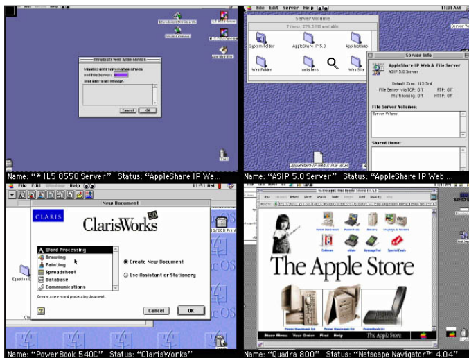
Apple Network Assistant lets you observe up to 250 remote computer screens. Screens appear four at a time in a rotating cycle.
